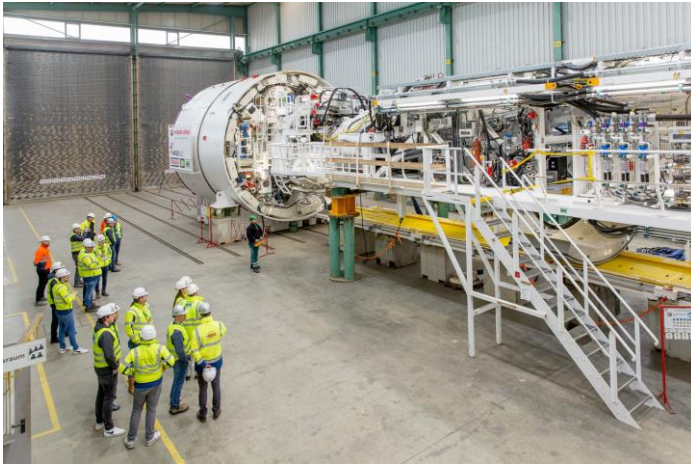
Factory acceptance of the new tunnel boring machine © Herrenknecht AG
